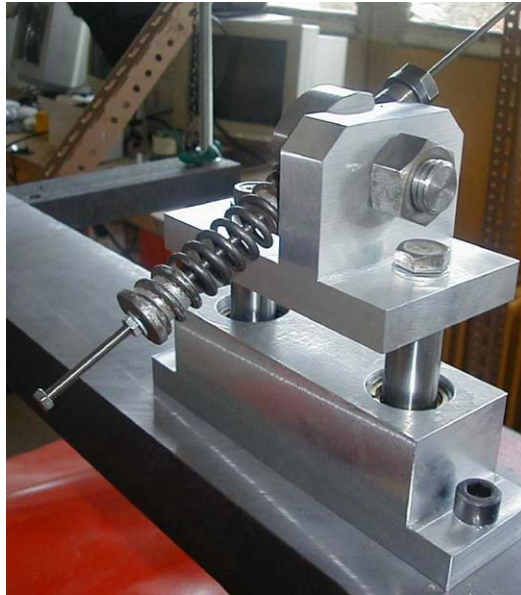
Fig. 3. Sub-system assembly with the stressing anchorage.
