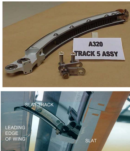
Fig. 2. A slat track (top) mounted in the wing of an Airbus320 aircraft (bottom).
