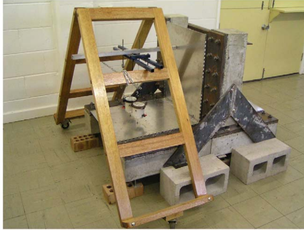
Fig. 2. Photograph of the T-shaped plate experimental rig, showing the primary and control shakers and the structural boundaries conditions.
