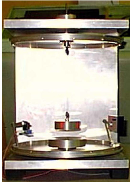
Fig. 1. Picture of the demonstrator built for the study of non-synchronous damping.
