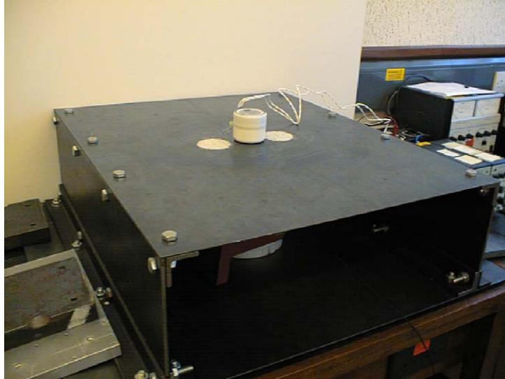
Fig. 15. The experimental arrangement, which consists of a finite flexible plate, driven by a primary force (shaker underneath), and controlled by a modified ULTRA Electronics inertial actuator placed on the flexible plate.
