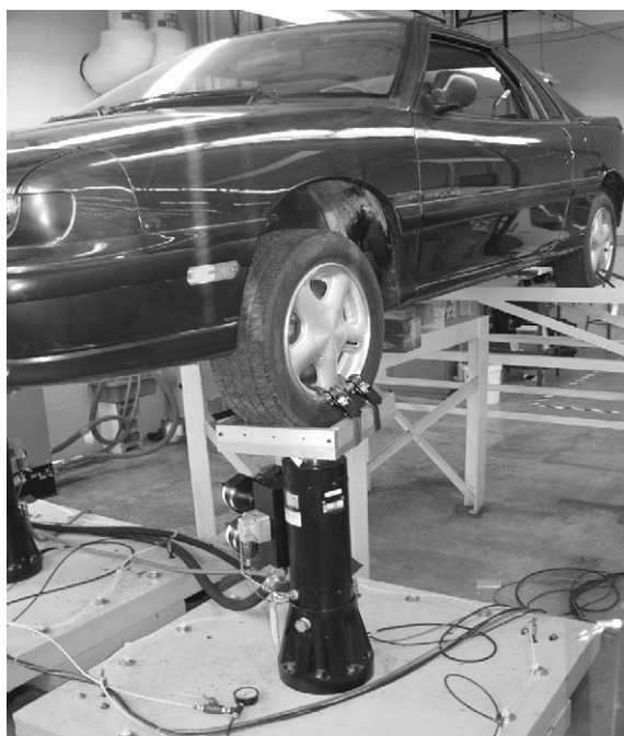
Fig. 6. Shaker testing setup with single corner of vehicle shown.
