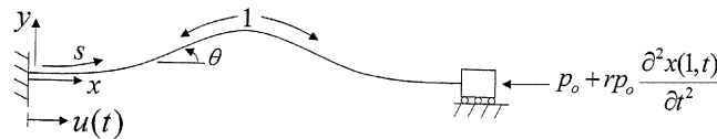
Fig. 1. Geometry of buckled or pre-bent column subjected to base motion and to static and inertia forces of supported weight, in nondimensional terms.
