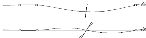
Fig. 15. Lowest mode shapes when the ER damper is treated as a bearing.
