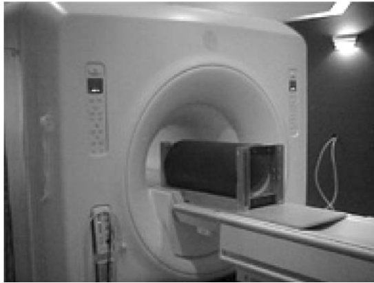
Fig. 1. The gradient coil installed in a 1.5T GE MRI.
