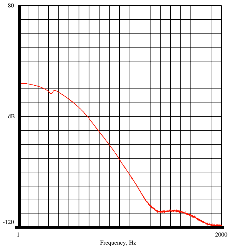
Fig. 4. A typical PSD of the impulse with hard tip.
