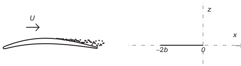
Fig. 1. Basic 2D problem with trailing-edge coordinates.
