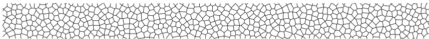
Fig. 1. A cellular beam. The microstructure is composed of irregular cells. Vibration in the plane of the paper is considered.
