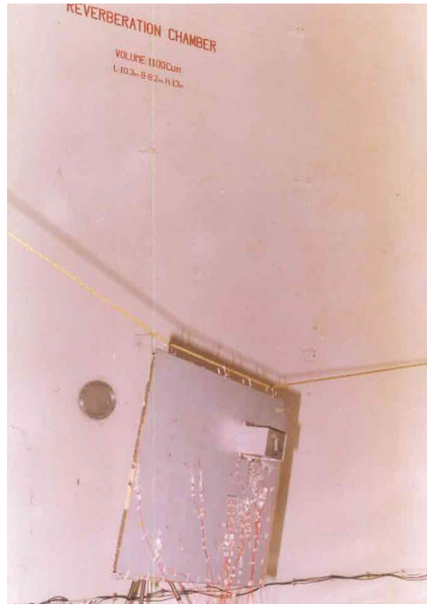
Fig. 2. Setup for the acoustic test on the panel with equipment.
