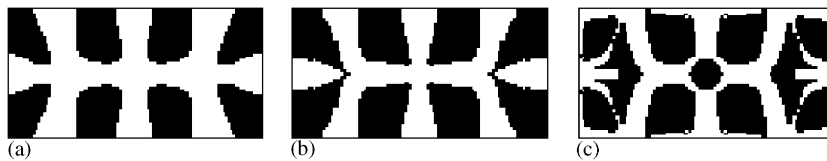
Fig. 12. Maximizing the separation of 7th and 8th eigenfrequencies ( n = 7 ). Compared to Fig. 11 the objective is here the ratio between the squared eigenfrequencies and the value of \alpha is changed but the value of \beta = 4.5 is kept fixed. (a) \alpha = 2 , \omega_8^2/\omega_7^2 = 2.12 , (b) \alpha = 4 , \omega_8^2/\omega_7^2 = 2.06 , (c) \alpha = 8 , \omega_8^2/\omega_7^2 = 2.00 .
