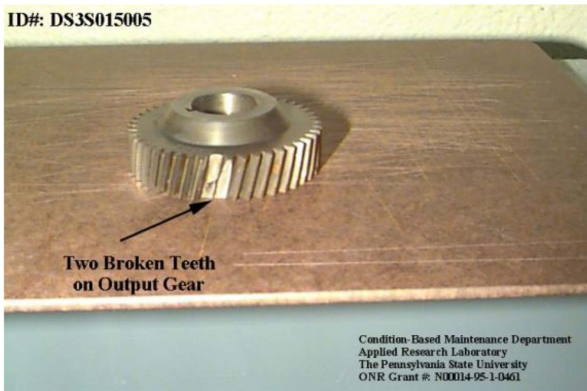
Fig. 4. Two adjacent gear tooth failures of the driven gear in test TR#5.
