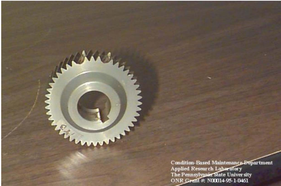
Fig. 8. Two non-adjacent gear tooth failures of the driven gear in test TR#8.
