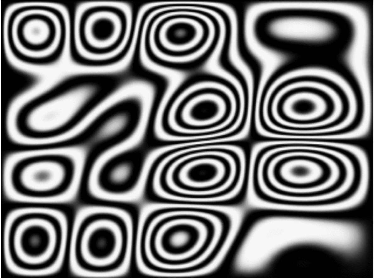
Fig. 4. Density plot of the real part of V_r(x, y, z_0, t) for the rectangular simply supported plate at t = 0.05 s.
