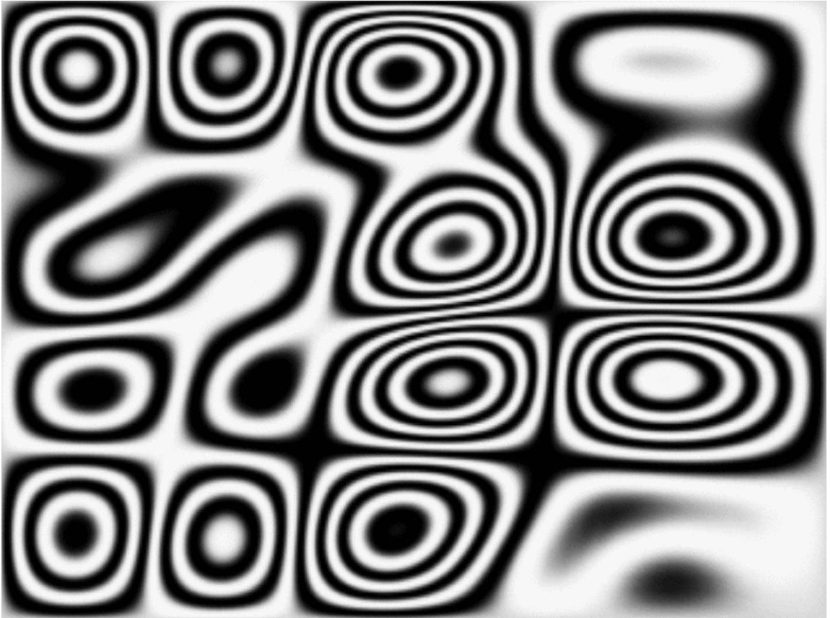
Fig. 5. Density plot of the imaginary part of V_r(x, y, z_o, t) for the rectangular simply supported plate at t = 0.05 s.
