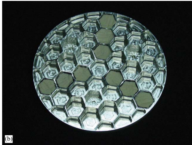
Fig. 7. Case study B with added damping along the radial direction and radial direction corresponds to smallest hexagon heights, 20 g added mass to overall structure.
