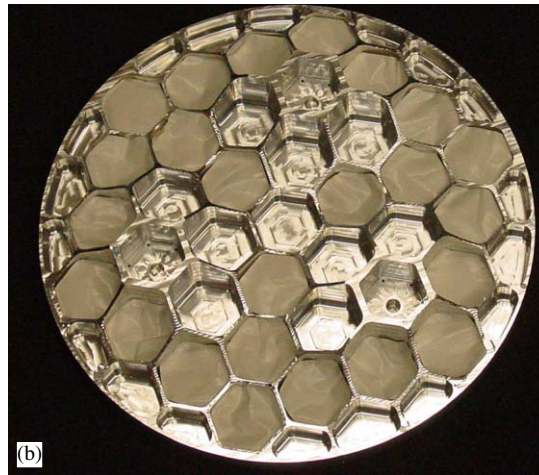
Fig. 8. Case study C with added damping along the radial direction (corresponds to smallest hexagon heights) and about the outer diameter, 53 g added mass to overall structure.
