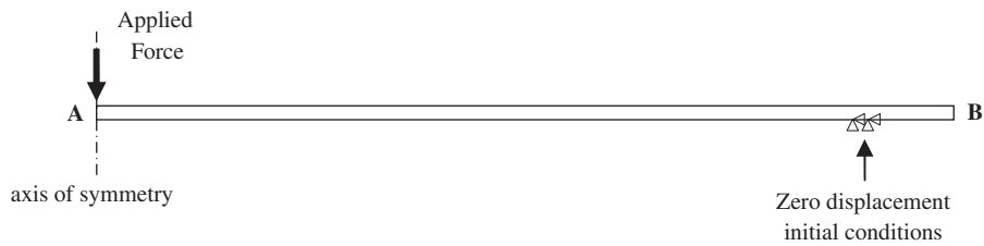
Fig. 11. The experimental set-up and the equivalent two-dimensional axi-symmetric FE model.
