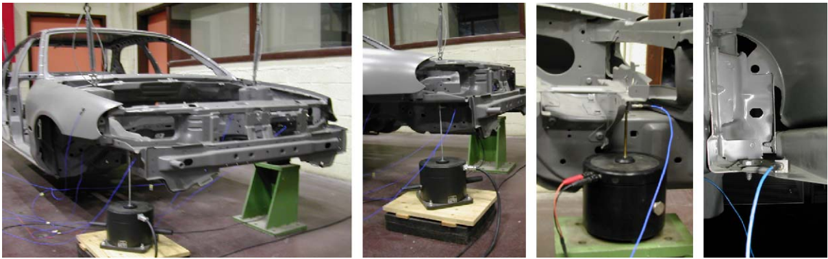
Fig. 4. Modal test setup for car body: (left) view on suspended car body, (middle) shakers applying dynamic loading to the car and (right) response sensor nearby a welded/screwed joint.
