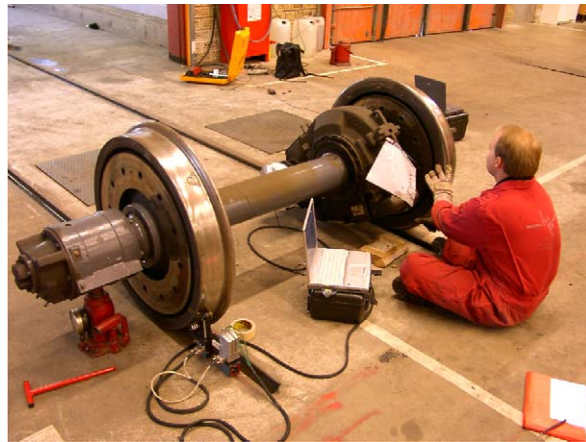
Fig. 2. Out-of-roundness measurement on a powered Regina wheelset.
