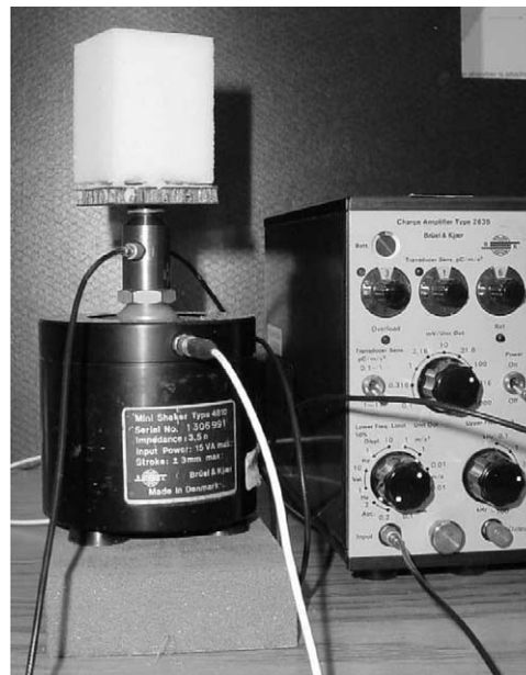
Fig. 3. Experimental set-up to measure inclusion apparent mass.
