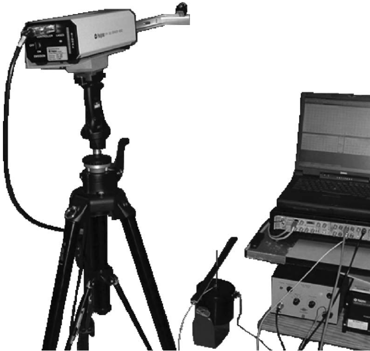
Fig. 5. Experimental setup for damping measurements.
