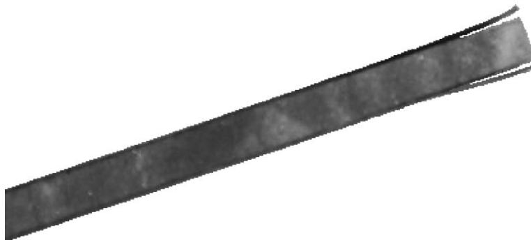
Fig. 4. A beam with 50.8 mm delaminations on both sides.
