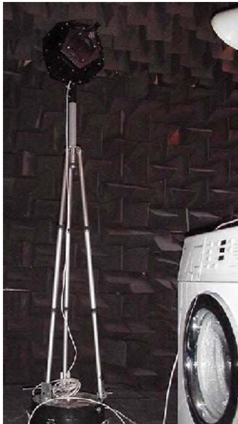
Fig. 11. Rotating dodecahedron loudspeaker use for reciprocal measurement of transfer functions.
