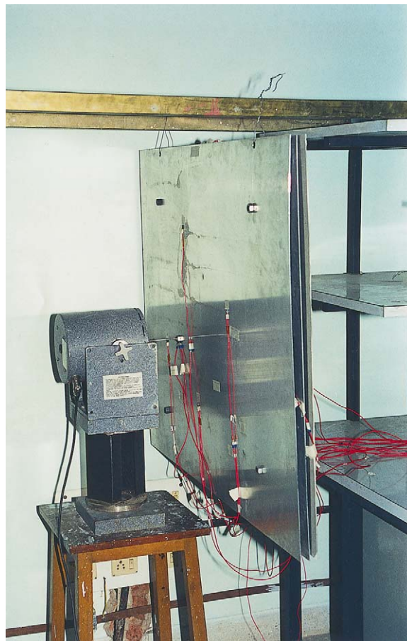
Fig. 4. Test setup for coupling loss factor measurement.
