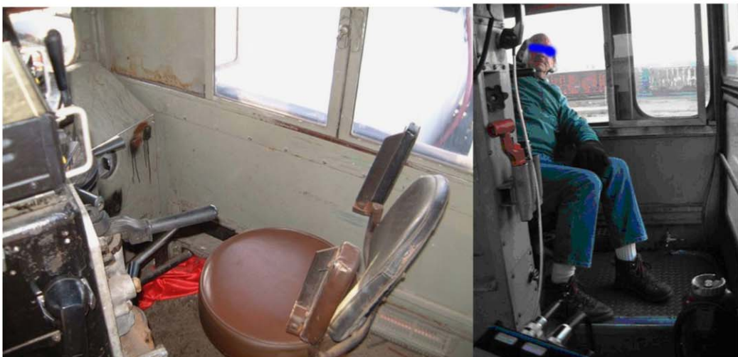
Fig. 1. Traditional cab and seat design (“American Standard Control Stand”), round toad stool, railroad engineer during yard switching.
