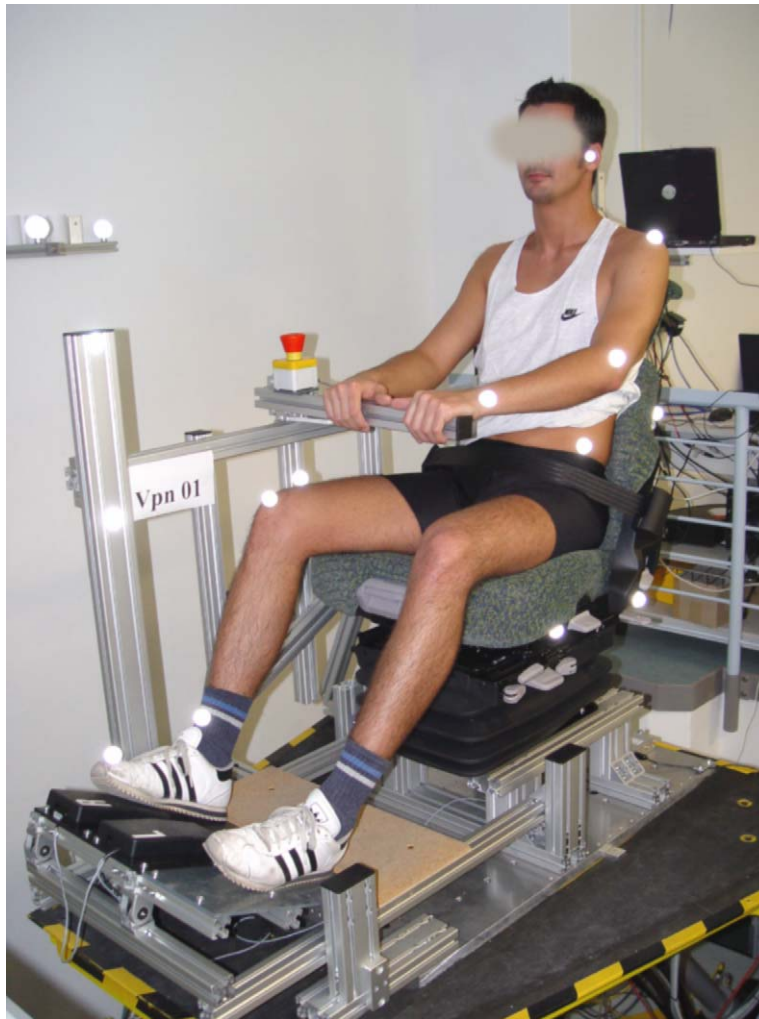
Fig. 5. Subject with applied markers for the motion analysis.
