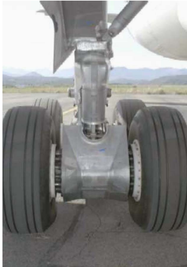
Fig. 6. Airbus A340 main landing gear equipped with fairings.
