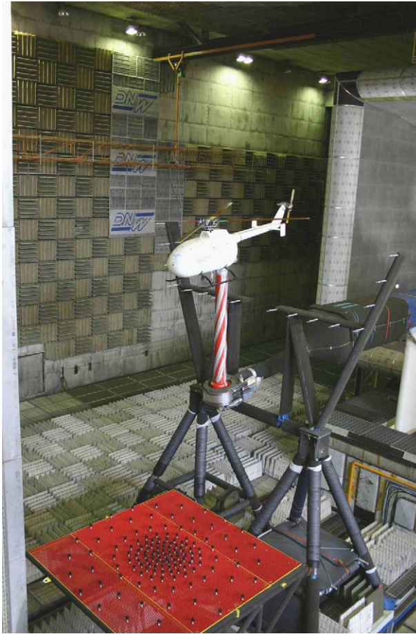
Fig. 30. HeliNOVI test set up for aeroacoustic test.
