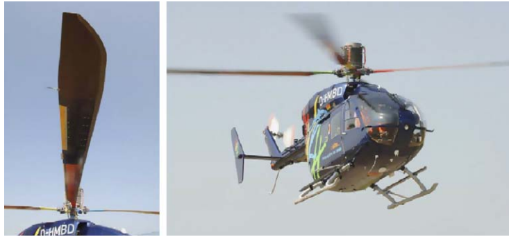
Fig. 29. Flight tests on a full scale helicopter equipped with blades using servo flaps for active blade control.
