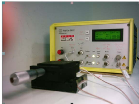
Fig. 1. The piezoelectric actuator system: a piezoelectric actuator stage with a built-in sensor (in the front), and a driving and sensing electronics unit (in the rear).
