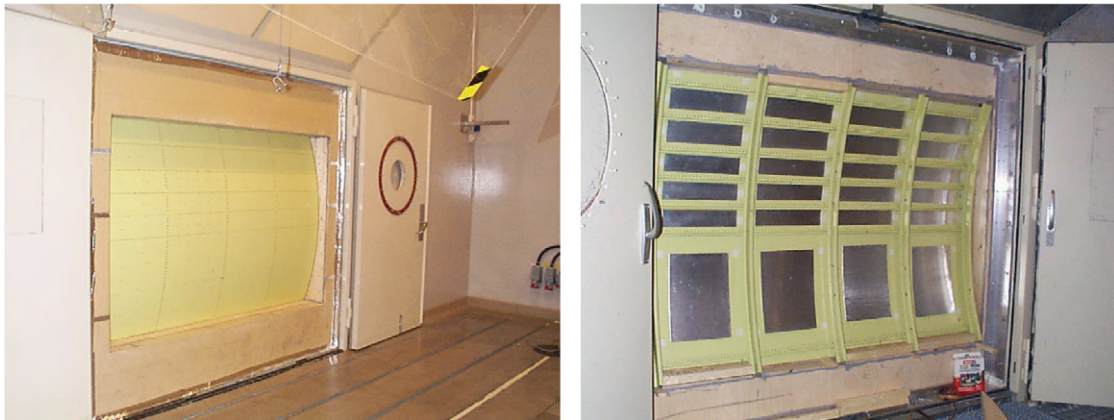
Fig. 10. Test arrangement for a large metallic panel (Panel G), (left), side of reverberation room, (right), side of anechoic room.
