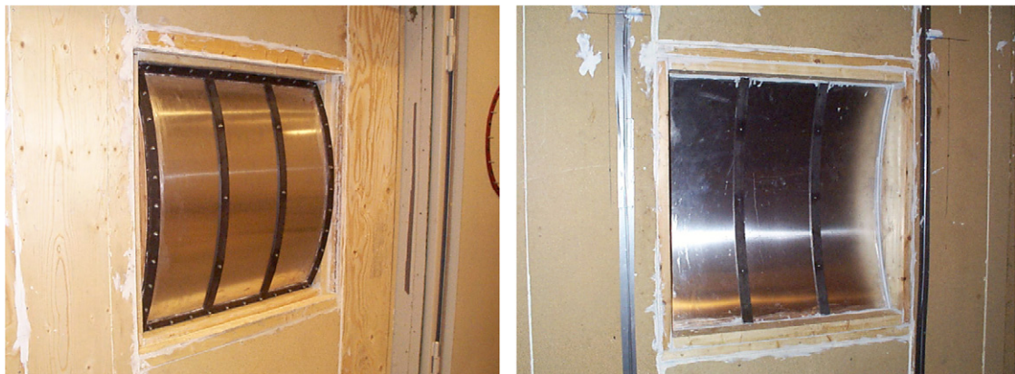
Fig. 8. Test arrangement for a home-made panel (Panel D), (left), side of reverberation room, (right), side of anechoic room.
