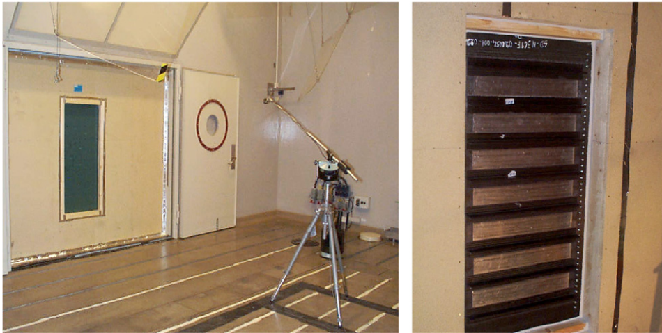
Fig. 9. Test arrangement for a small aircraft panel (Panel F), (left), side of reverberation room, (right), side of anechoic room.
