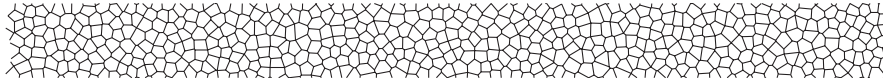
Fig. 1. A cellular beam made of irregular cells. The beam vibrates in the plane of the paper.
