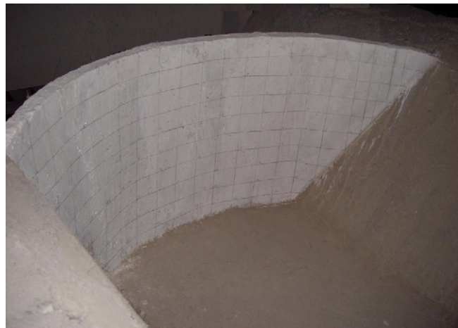
Fig. 2. Experimental model of the arch dam.
