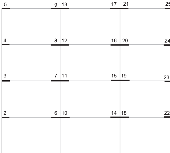
Fig. 4. The material numbers for the damaged elements in the FE model of the reinforced concrete frame. Materials numbers 2 to 25 represent the damaged elements whose stiffnesses will be updated. Material number 1 corresponds to the undamaged elements.
