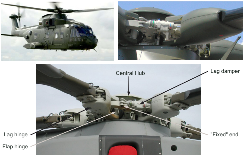
Fig. 1. Close-up of the EH101 hub rotor system.
