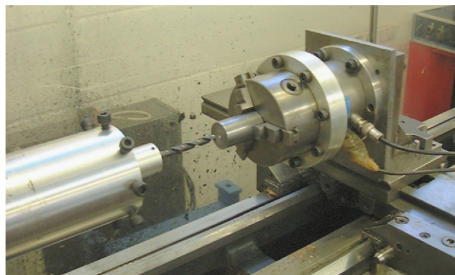
Fig. 7. Experimental arrangement for drilling reaction force/torque measurement.
