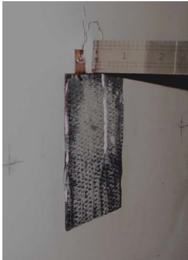
Fig. 6. Viscoelastic constrained layer-damping material (3 M 112P05).
