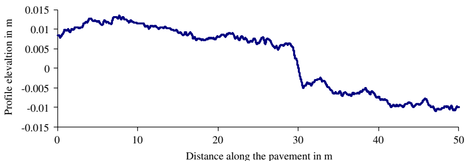
Fig. 3. Artificially generated good surface profile (profile 0, provided as an example for the road profiles mentioned in the paper).
