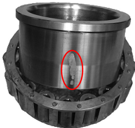
Fig. 16. Bearing with localized inner-race defects.
