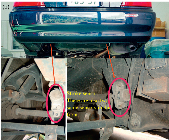
Fig. 8. Experimental system: (a) control system and data acquisition architecture, (b) stroke sensor and (c) G sensor.
