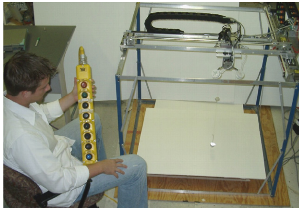
Fig. 14. Portable bridge crane.
