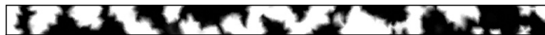
Fig. 3. Optimized design for the rectangular room for the higher target frequency f = 4 \times 34.56 Hz.
