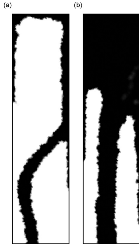
Fig. 13. The optimized designs for the target frequency f = 63 Hz: (a) with volume fraction \beta = 0.24 and (b) with volume fraction \beta = 0.9 .
