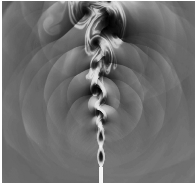
Fig. 24. 2D simulation of a jet, including the mach discs, vortices and the acoustic waves.
