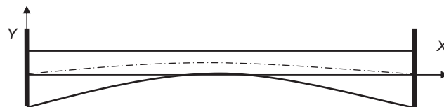
Fig. 7. General non-uniform and non-circular curved beams representing an overpass bridge.
