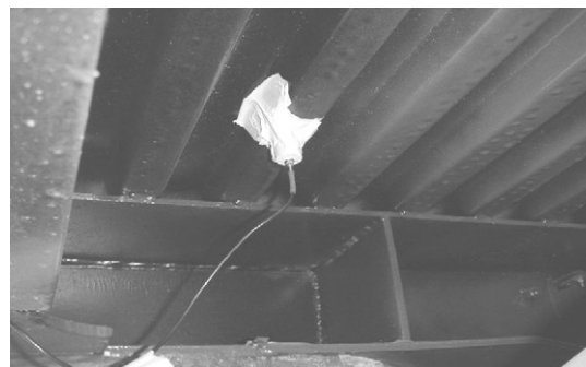
Fig. 6. Schematic diagram of the accelerometer location 7 under the vehicle floor.
