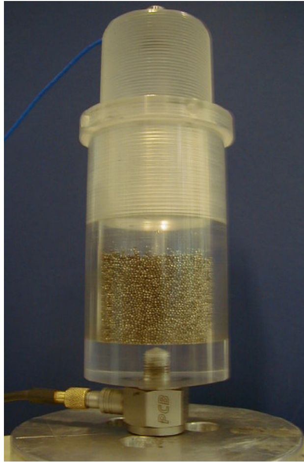
Fig. 13. Installation of the Perspex casing on the shaker for vertical excitations.
