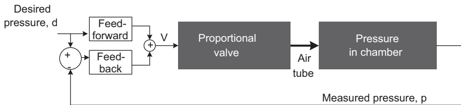
Fig. 9. Block diagram to control pneumatic pressure in chamber by both feedforward and feedback control.
