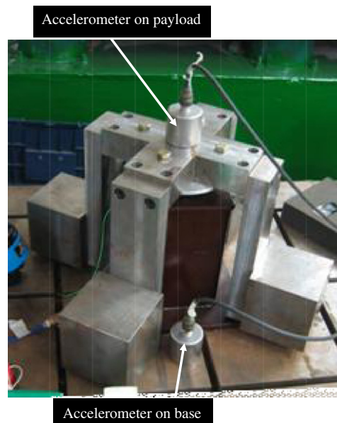
Fig. 13. Experimental set-up to measure transmissibility for base excitation.
