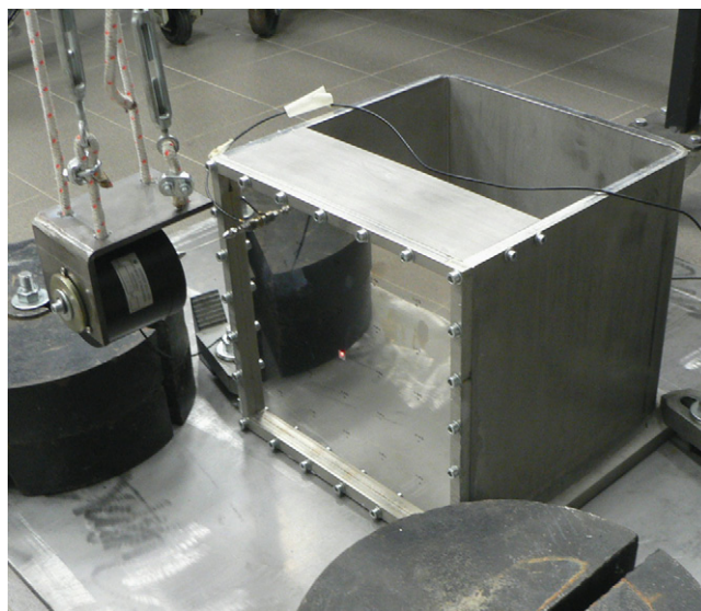
Fig. 1. Photo of the stainless steel thin rectangular plate fixed to a thick frame with a traditional exciter (shaker) and laser spot at the centre of the plate.
