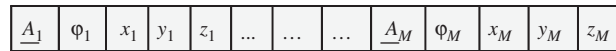
Fig. 4. Representation of a chromosome used for equivalent source method with the genetic algorithm (ESGA).
