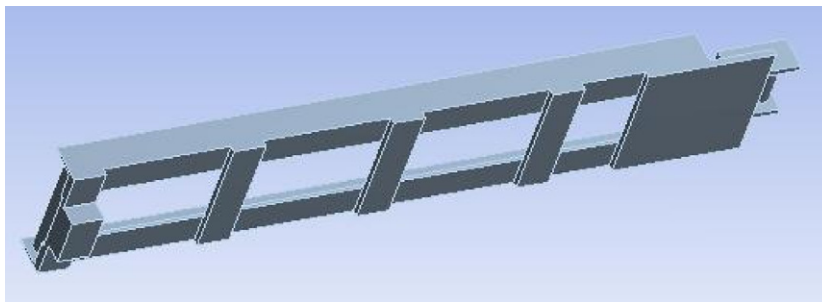
Fig. 14. A frame with mass 0.942 kg in the middle of the end member (left in the picture) of the structure.
