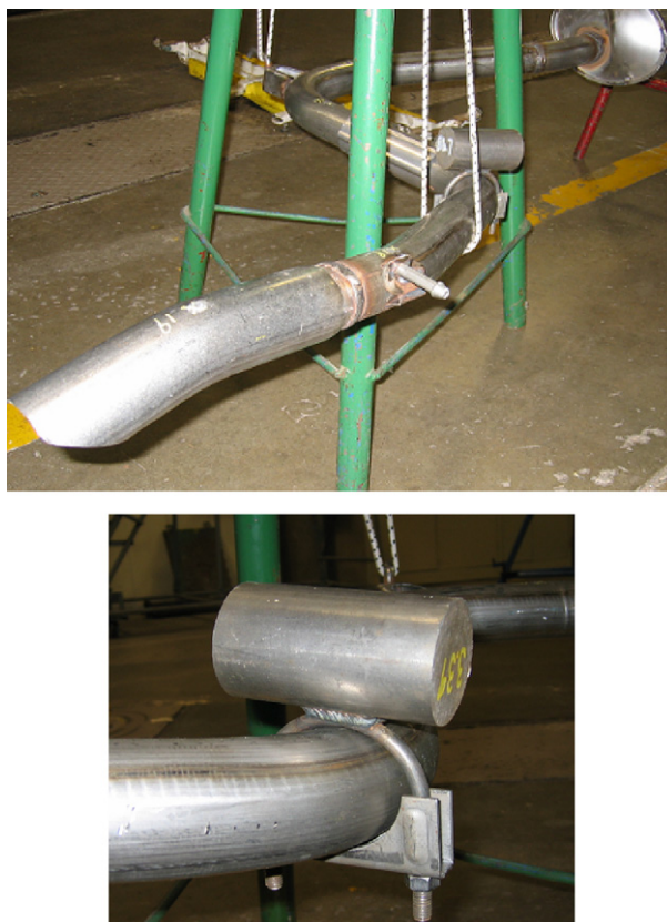
Fig. 20. An exhaust system tested for reduction of vibration at engine idle and lumped mass attached to the system.
