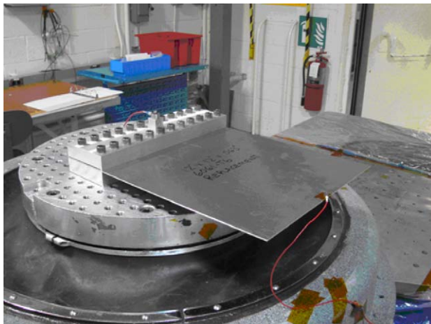
Fig. 4. Photograph of shaker table with square aluminium plate mounted in test position.
