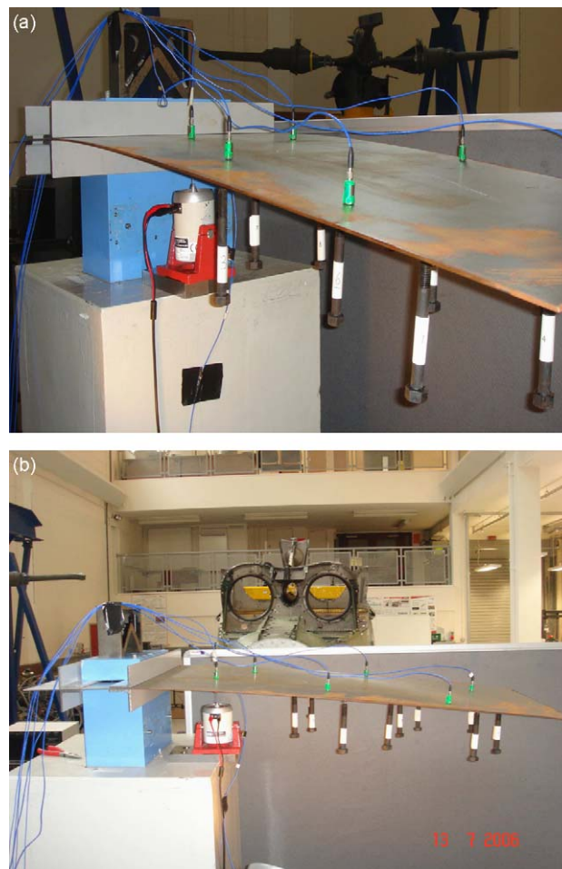
Fig. 1. The test rig for the cantilever plate: (a) front view of the experimental setup and (b) side view of the experimental setup.
