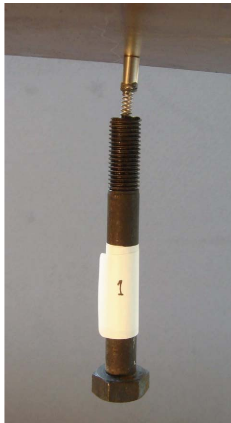
Fig. 2. Details of a typical oscillator used to simulate unmodeled dynamics. Fixed mass (magnet) 2 g, oscillatory mass (the bolt) 121.4 g. The oscillatory mass is about 1% of the total mass of the plate. The spring stiffness varies between 1.5 and 2.4 \times 10^4 N/m.
