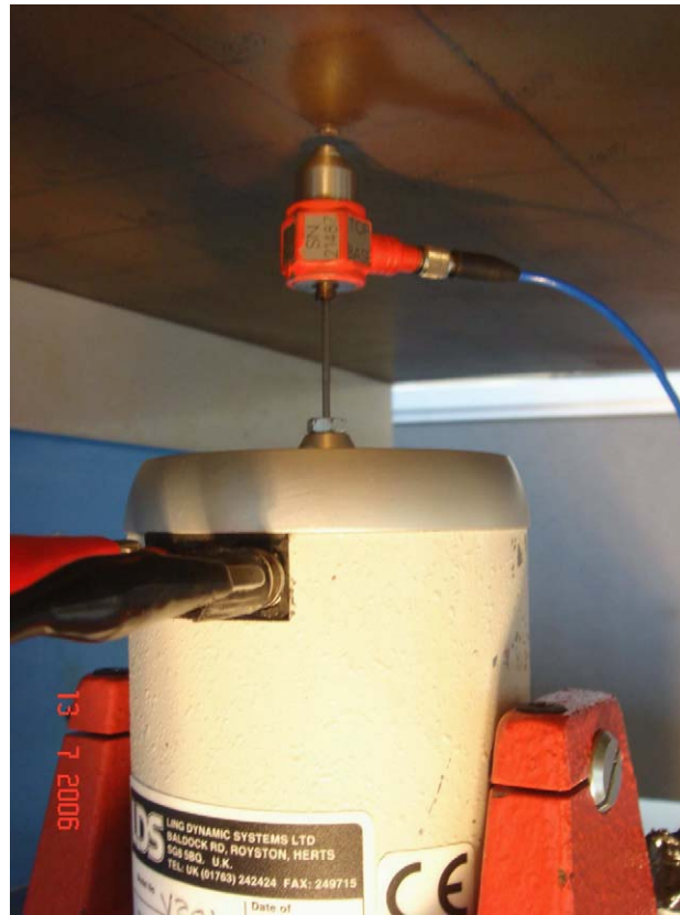
Fig. 4. The shaker used to provide an impulse excitation using Simulink™ and dSpace™. A hard steel tip was used and the shaker was placed at node (4, 6).
