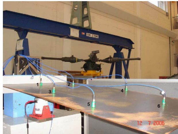
Fig. 5. The positions of the accelerometers on the plate.
