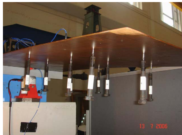
Fig. 3. Attached oscillators at random locations. The spring stiffness varies so that the oscillator frequencies are between 43 and 70 Hz.
